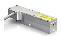
For generating high peak power IR pulses of a few hundred picoseconds, microchip lasers are economical, compact, and reliable. Sub-nanosecond 1064nm pulses are indeed directly generated from the diode pumped passively Q-switched Nd:YAG microchip engine.
