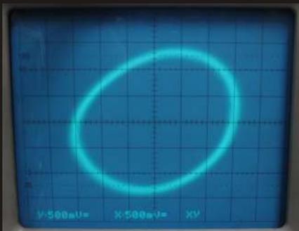
a) IQ (quadrature) mixer output (while unlocked)
