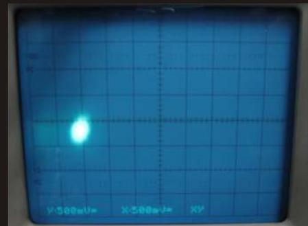
c) IQ (quadrature) mixer output when locked
