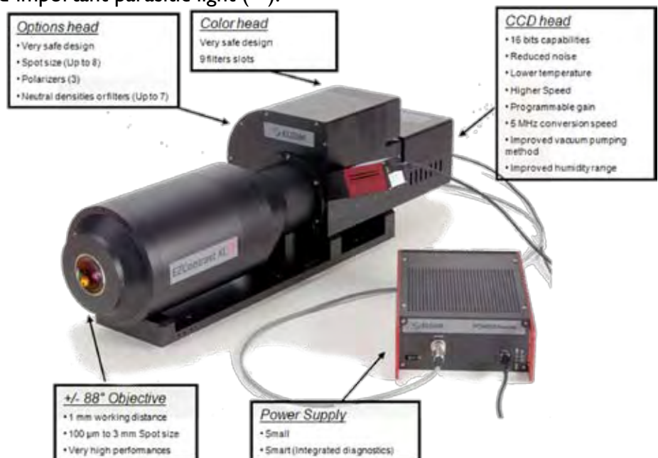
Description of the EZContrastXL88 with its main components
