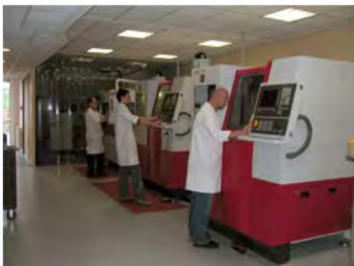
CNC (Computer Numerically Controlled) systems for grinding, polishing and centering
