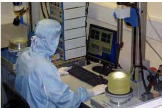
Lens alignment in clean room
