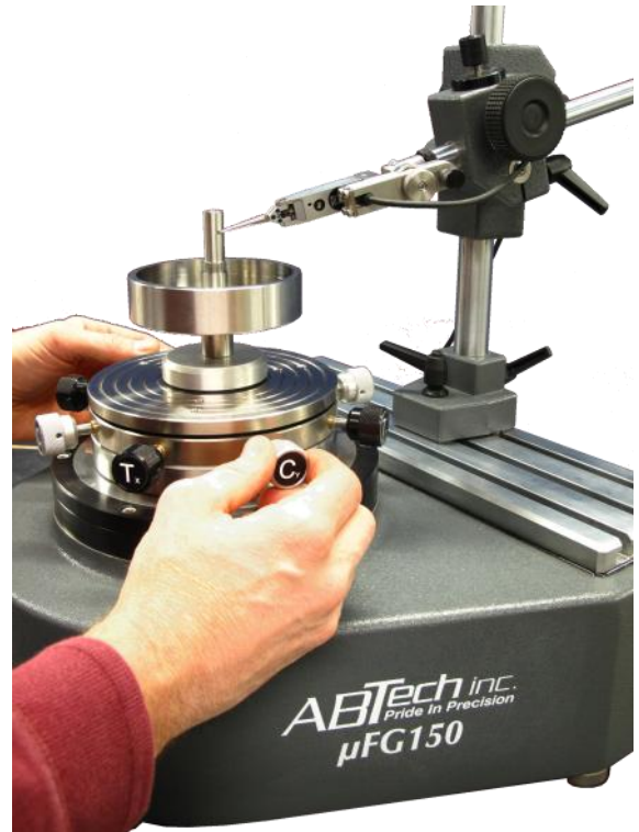
Fine action for leveling and centering the part with ABTech's spherical seat tip/tilt design. Lock in the adjustments using eight opposing knobs to eliminate hysteresis and provide superior position stability.
